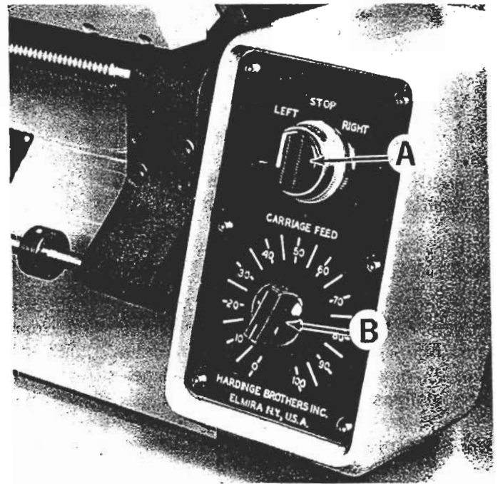
Figure 13 — Power Feed Control Box
